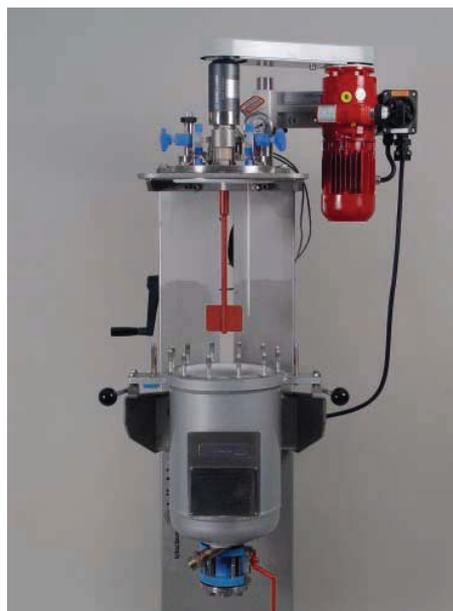
With tiltable lowering device for easy cleaning and maintenance.
