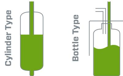
The Swagelok grab sampling systems provide solutions to satisfy gas and liquid non-slurry sampling service in a consistent, reliable package. Two system types allow for capture into one of two types of containers — pressure-containing metal cylinders as found in the Grab Sample Module (GSM) or non-pressure-containing glass or polyethylene bottles as found in the Liquid Only Sampling Module (GSL).
