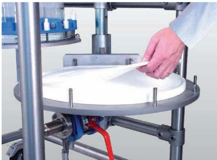
Exchange and cleaning of the filter.
