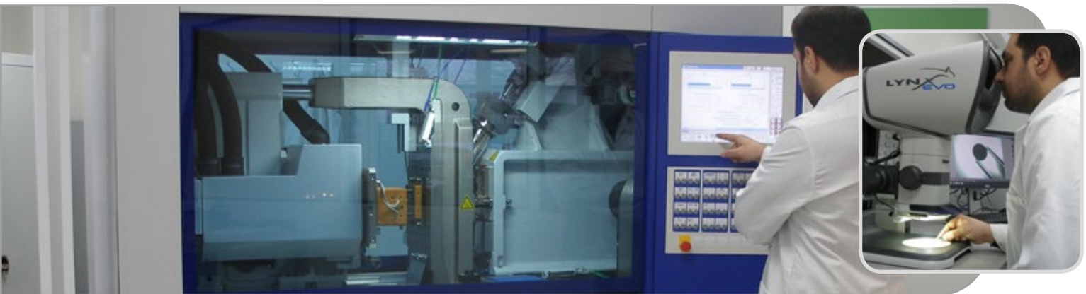
MicroForm® fully automated manufacturing cell (ISO Class 6 environment)
