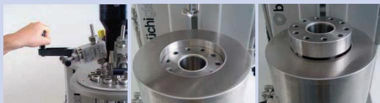
Manual lift for lowering the electric heating.
