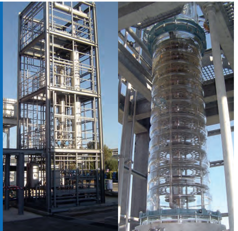
DN400 liquid/ liquid extraction column capacity 800kg/h
