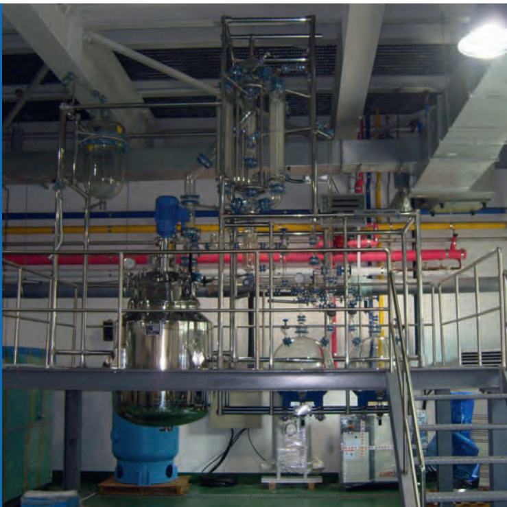
1000 liter cryogenic reactor with glass upper section
