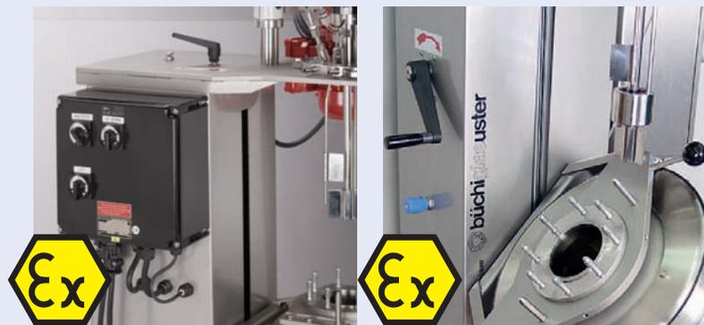
kiloclave with electrically driven lift
