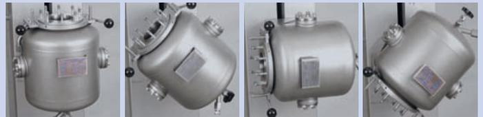
Pivoting function for easy vessel cleaning
