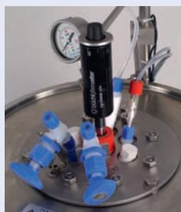
Cover plate with 6 openings and accessories made of PTFE, PFA, PEEK or glass
