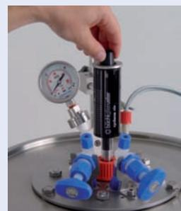
Integrated motor with speed control
