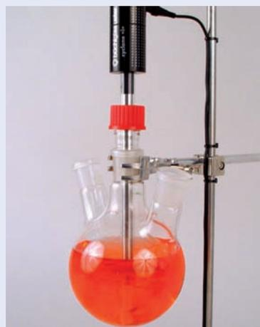
Installation of cyclone «i» with NS29/32 on round flask.
