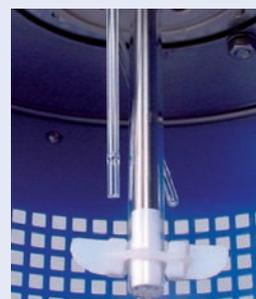
PEEK cover plate from inside with dip tube, Pt100-sensor and stirrer
