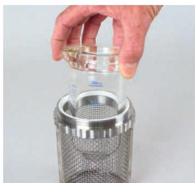
Vessel holder with protective wire mesh
