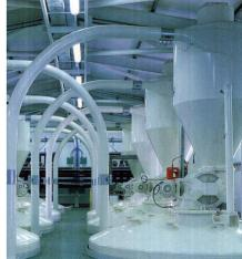
Above: Low velocity conveying system for the gentle handling of tea blending system.
