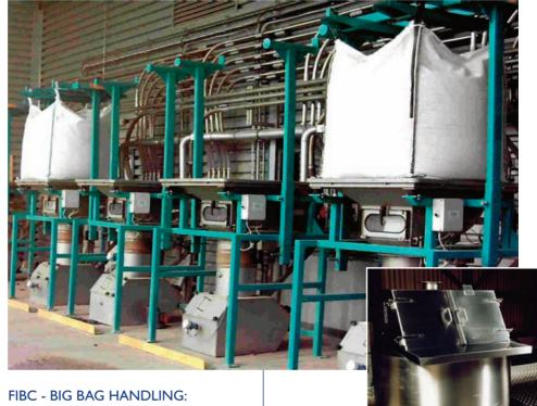
STB have designed a technically advanced range of big bag discharge and filling systems. Each system provides a means of safe handling I tonne big bags with dust free discharge and filling.
