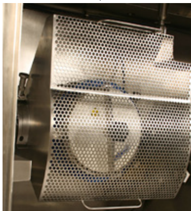
Interlocked glove guards provide safety during contained blending.
