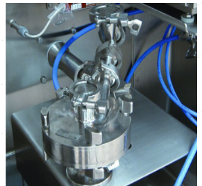
Integrated Feeder and Micronizer Jet Mill
