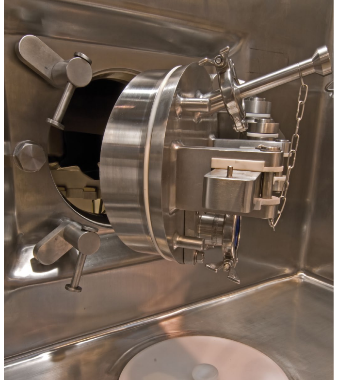
Discharge hatch with sampling port including high containment product offload and heel recovery gloveboxes designed and integrated by PSL
