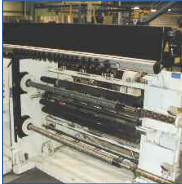
A new rewind unloading system fitted to a Titan SR5 slitter rewinder increases production
