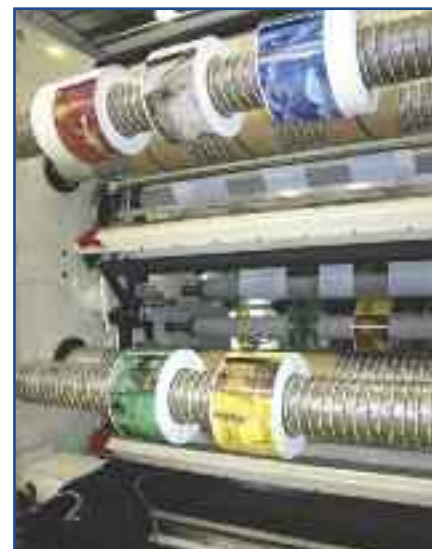
152 mm / 6 ins Quick Shafts on a turret rewriter
