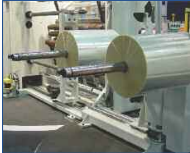
Unloading booms reduce rewind package handling
