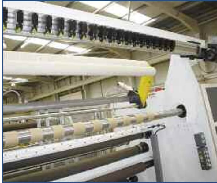
Laser core positioning system above rewind shaft
