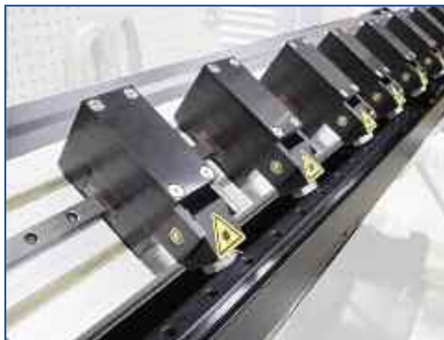
Lasers improve roll alignment
