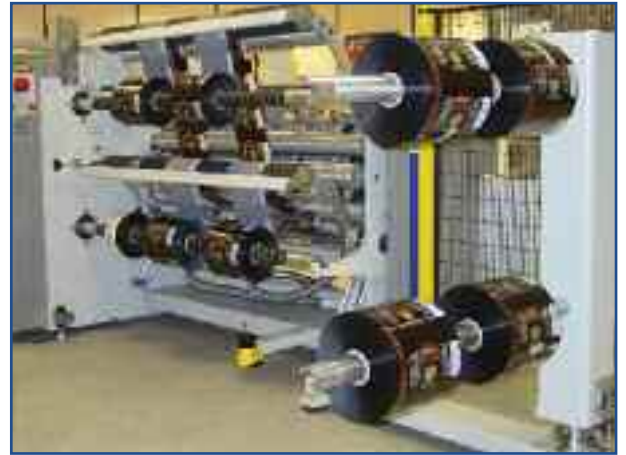
Slit reels unloaded to boom
