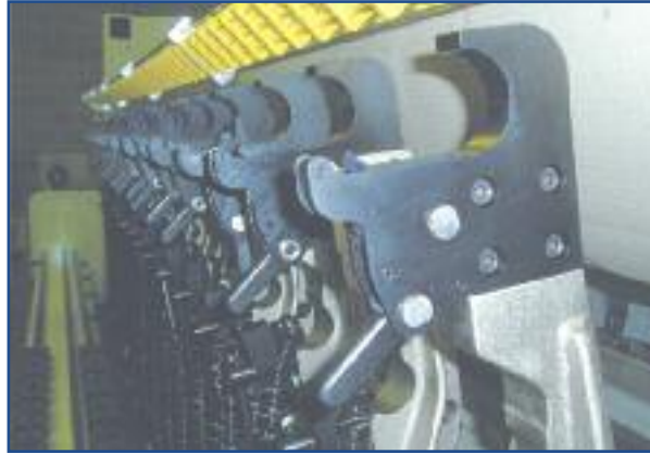
Quick-release contact roll clamping mechanism
