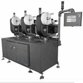
The very latest requirements are incorporated in the new range of Print and Apply equipment from Cobalt Systems. Real time data management determines label design and content for every label at the point of printing. The label printed is the label applied, with secure procedures to optimize barcode quality, printed to the highest standard ensuring compliance and successful application to the pack.
