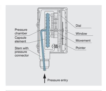
Fig. Pressure gauges with capsule elements
