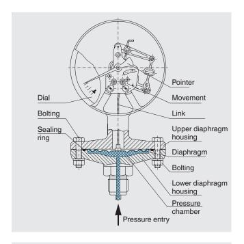
Fig. Pressure gauges with diaphragm elements
