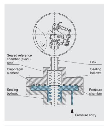
Fig. Absolute pressure gauges
