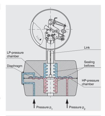
Fig. Differential pressure gauges
