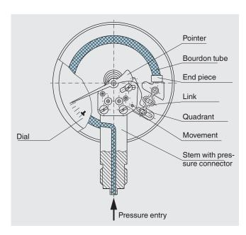
Fig. Pressure gauges with bourdon tube
