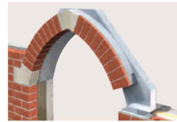
Isometric view showing IG's Gothic Arch BSFL. Upon request the box frame, which the bricks are fixed to, will stop short of the end bearing of the lintel. This allows quoin stones to be placed into position onsite.
