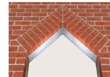
View showing the underside of IG's Apex BSFL. This illustrates how the brickwork returns under the soffit of the lintel to ensure no steelwork is visible on the outer leaf.
