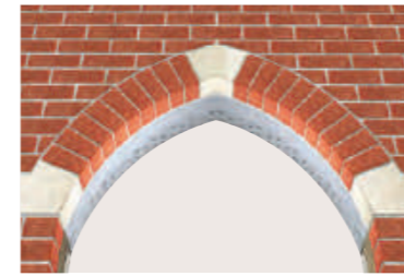
View showing the underside of IG's Gothic Arch BSFL. This illustrates how the brickwork returns under the soffit of the lintel to ensure no steelwork is visible on the outer leaf.
