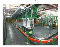
This system can also reduce / eliminate costly downtime due to weigher malfunctions as each weigh carriage can be simply removed from the track for maintenance or repairs. The remaining carriages will then continue the weighing operations or an additional spare carriage can be added to maintain the same throughput.
