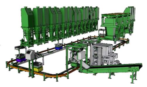
Each carriage incorporates a high accuracy force motion platform scale to give typical weighing accuracies on minor ingredients of +/- 3g or better. As the smart cart carriages run upon a continuous monorail track numerous carriages can be added to increase overall throughput.
