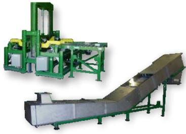
Bespoke system for a Spanish polymer processing company. These two machines were supplied as part of a complete polymer recycling plant. Machine 1 accepts 1M3 polymer blocks, cuts off 1" slices, lowers the slice down then takes it back through the guillotine to create 1" x 1" strips. Strips are then rotated and cut into cubes. Machine 2 accepts feed of cubes into water bath before elevating them and discharging to the downstream drying system.
