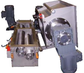
For applications where higher batch sizes and varying throughputs are required specialist feeders can be supplied which include duplex flights of different diameters to increase throughput range whilst maintaining accuracy. For maximum throughput both flights are run simultaneously and for maximum accuracy just the smaller flight is run.
