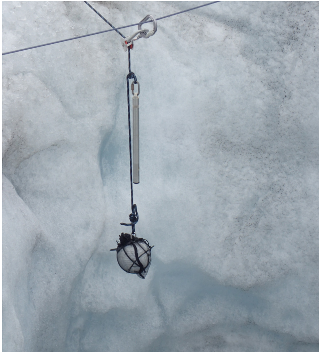
The Cryoegg is attached to a rope and lowered into the moulin
