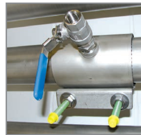
B Spot drilling collar
