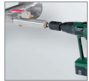
Drill under pressure with the CS Drill
