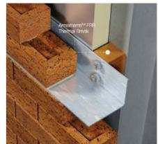
To improve the U value of a masonry wall assembly, the shelf angle can be connected to the structure at discreet, evenly spaced points such as plate "blades" allowing the insulation to pass behind the steel angle, reducing the effects of a continuous thermal bridge. However, building the shelf angle outwards requires larger geometries and additional material to support the cantilevered load.
