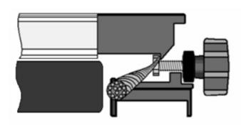
Tighten the knob to secure the bolt head against the wire.
