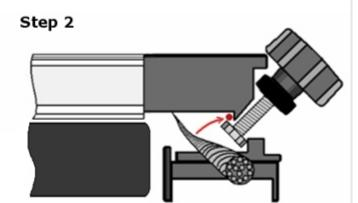
Using the knob, push the bolt in and tilt upwards to allow the wire to fit behind the bolt head
