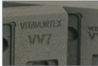
Laser etched ID in foam
