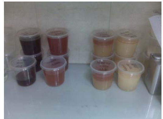
Separate water from recovered plasticiser for re-use
