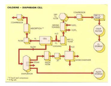
When the Chlorine gas leaves the Diaphragm Cell, it is cooled and then dried in a Drying Tower by contact with Sulphuric Acid. Before the chlorine gas is dried Wet Chlorine filters should be installed.
