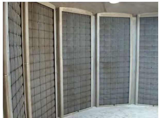
Inside View of Vertical Demister Panel Polygon
