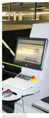
The Universal Fuzion automates odd-form component assembly increasing repeatability and quality
