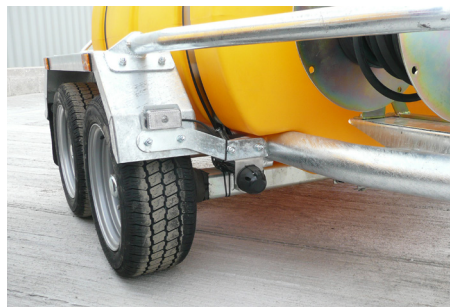
SIDE REFLECTOR AND TRAILER LIGHTING CONNECTION
