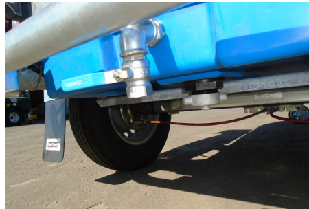
1" OUTLET AT FRONT AND REAR
