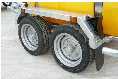
GALVANISED MUDGUARDS WITH SIDE REFLECTORS
