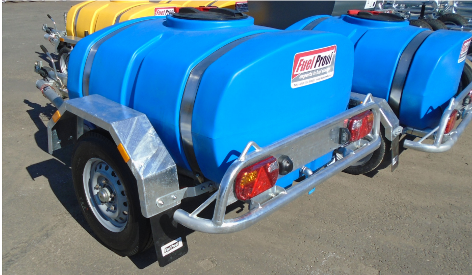
HIGHWAY TOW WATER BOWSERS FEATURE GALVANISED MUDGUARDS AND REAR LIGHTING BOARD
