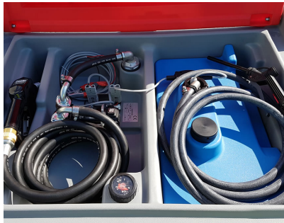
DUAL DIESEL / ADBLUE DISPENSING SYSTEM - (ON 400 + 50L TANKS)
