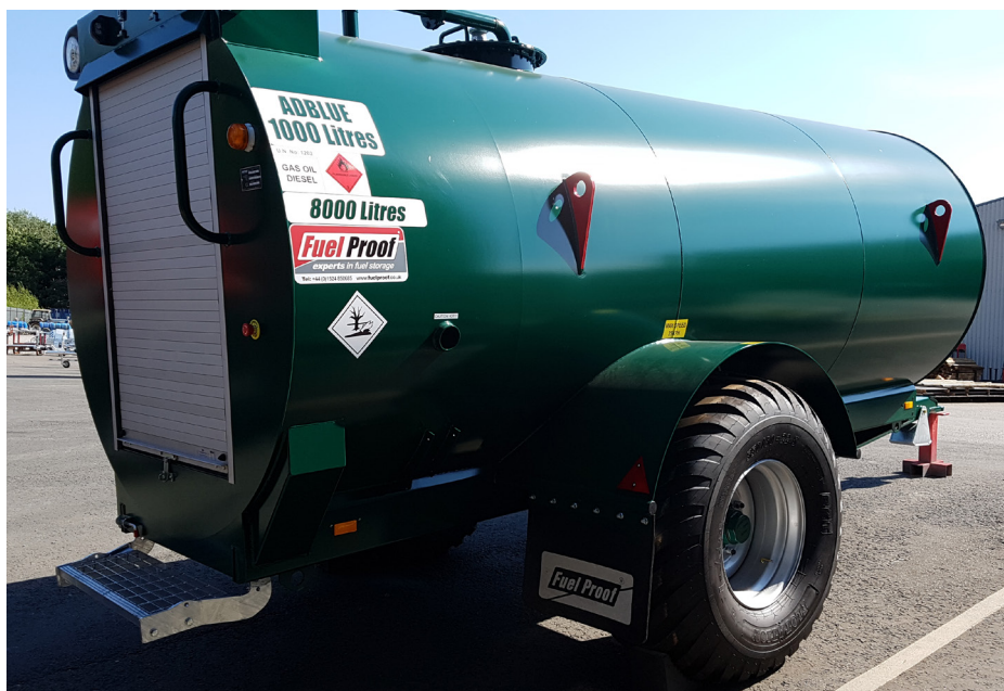
8000 LITRE SITE DIESEL BOWSER C/W 1000L ADBLUE TANK
