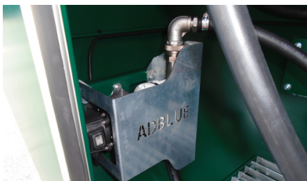
STAINLESS STEEL ADBLUE TANK / LOCKABLE DOOR
