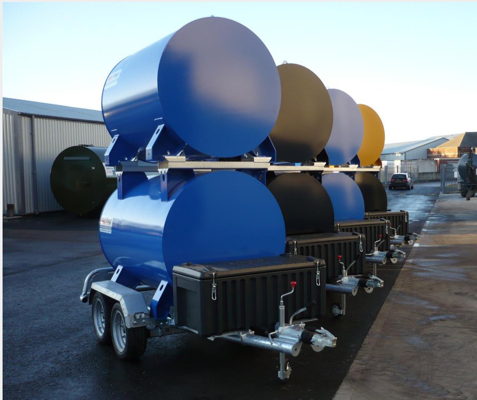
1,000 LITRE DE-MOUNT IBC'S STACKED ON HIGHWAY TOWABLE CHASSIS (TOOLBOX OPTIONAL)
