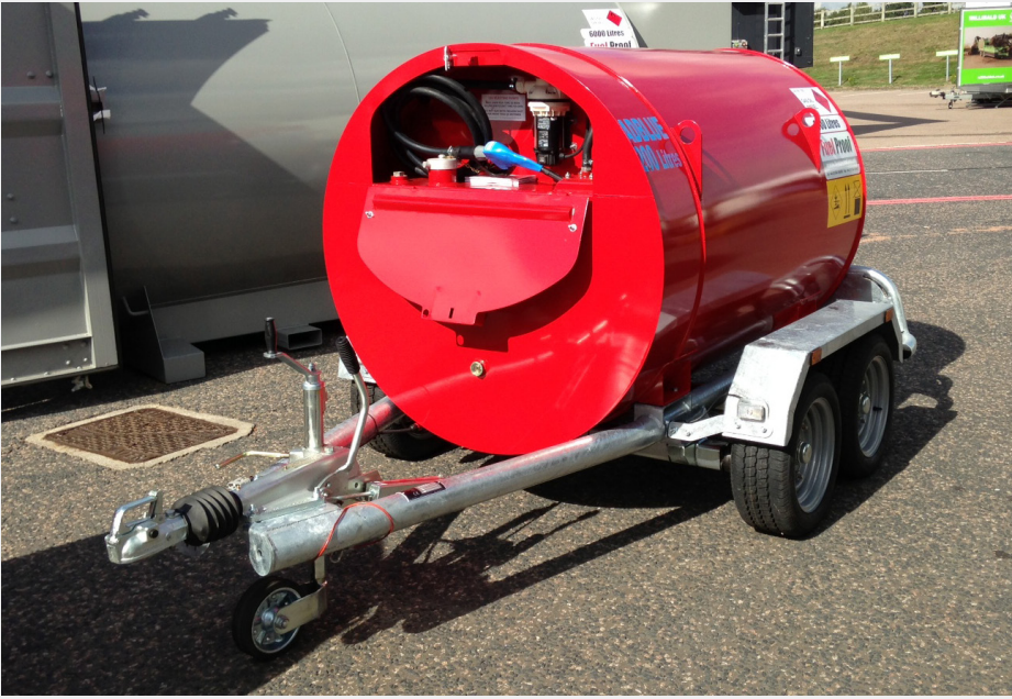
1000 LITRE HIGHWAY DIESEL BOWSER C/W 200L ADBLUE TANK
