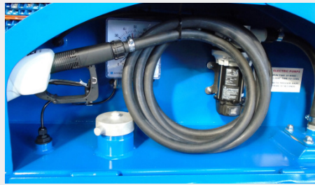
ADBLUE DISPENSING EQUIPMENT / ADBLUE FILL POINT
