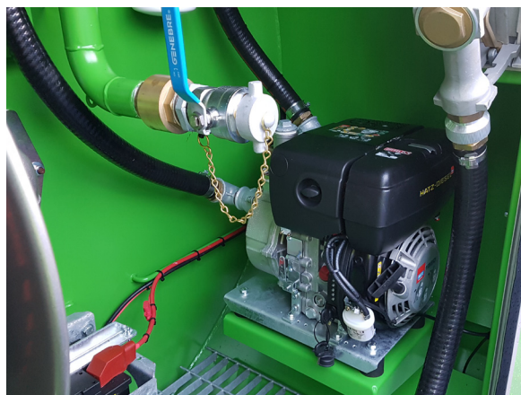
HIGH FLOW DIESEL ENGINED PUMP OPTION ON DIESEL TANK
