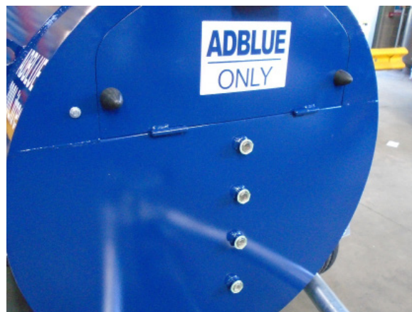
4 X SIGHT GLASS ON ADBLUE TANK FOR LEVEL READING
