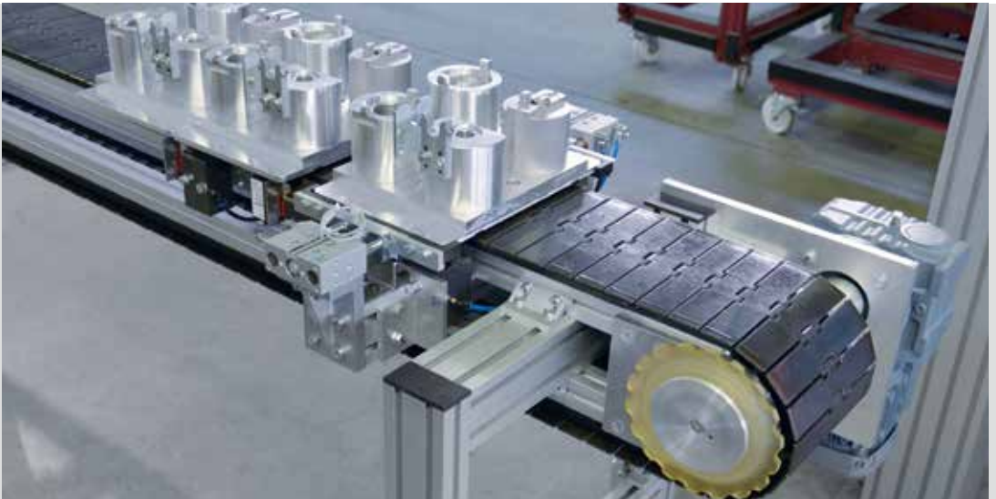
SPU with separation function for manual loading and robotic removal
