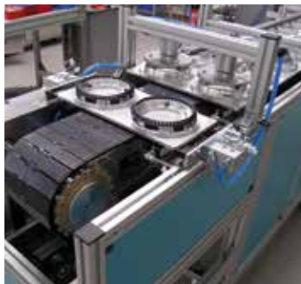
SPU System 190 with pallet for two workpieces
