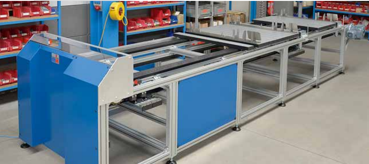
SPU double-lane system with separation function for supplying components to an assembly and welding machine
