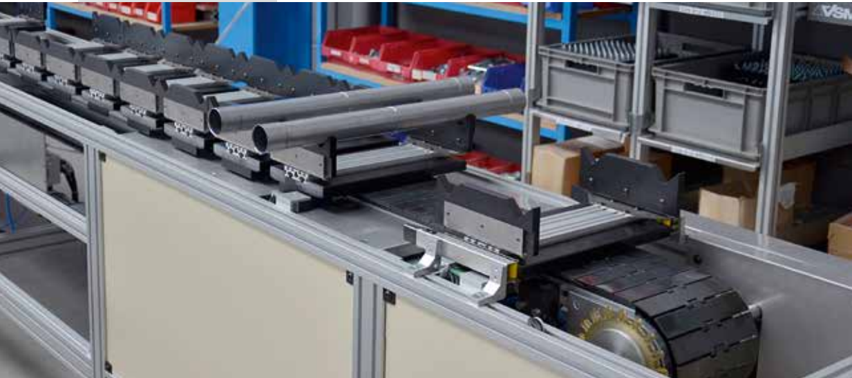
Accumulating pallet recirculation system with automatic pallet separation function designed for supplying components to a production process
