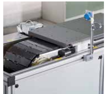
SPU with separation function for manual removal during continuous operation
