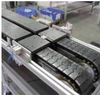
Centering unit for precise positioning of the workpiece carriers
