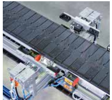
Centering unit for separation and stopping
