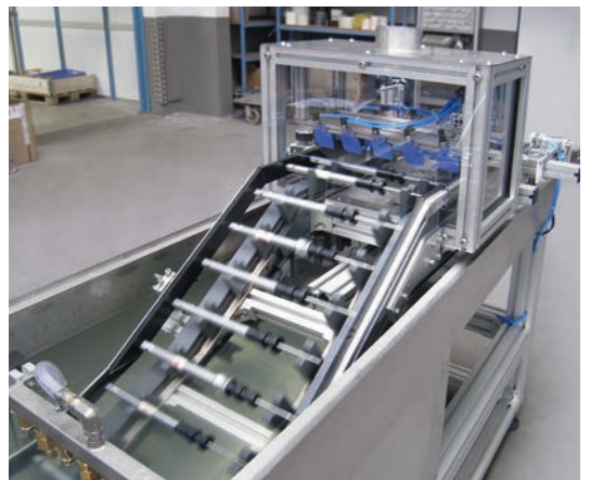
Customer-specific TKU 2040 with 20° inclination and transport of workpieces through a cleansing bath
