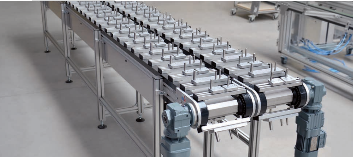
Double-conveyor system with order-specific profile pallets and fixtures
