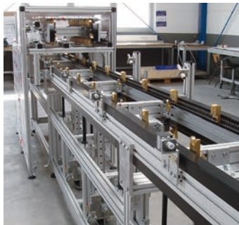
TKU 2040 with extractor unit and conveyor for rejected pieces
