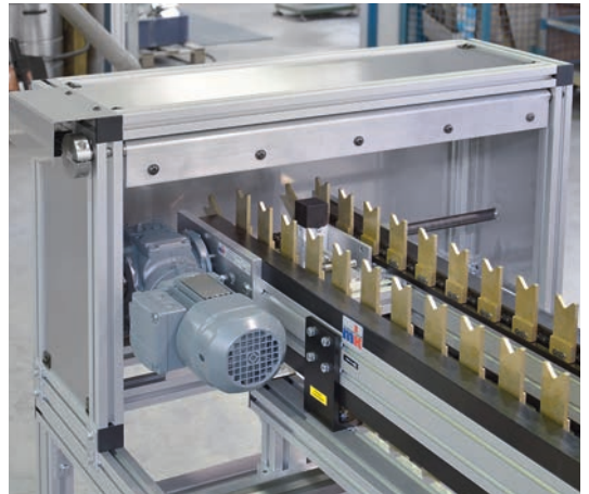
TKU 2040 with protective device guard on the drive side
