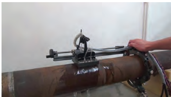
Chain Phased Array Crawler (XY axis)
