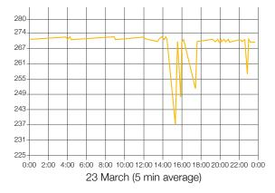
This graph clearly shows the battery voltage discharge and recovery as the charger returns after each mains failure.
