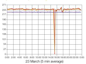
The input voltage data on this graph clearly shows the first major power cut. The output voltage is unaffected and steady on all 3 phases throughout.
