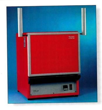
The heated chamber is formed from hard-wearing sillimanite and is located within the one piece outer case, an air gap and a graded selection of the latest high efficiency light-weight insulation between chamber and case achieves both a high thermal efficiency and cool outer case.
