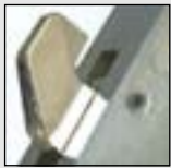
Hook - Anti-separation device. Locks in either an upward or downward direction and secures behind striker.
