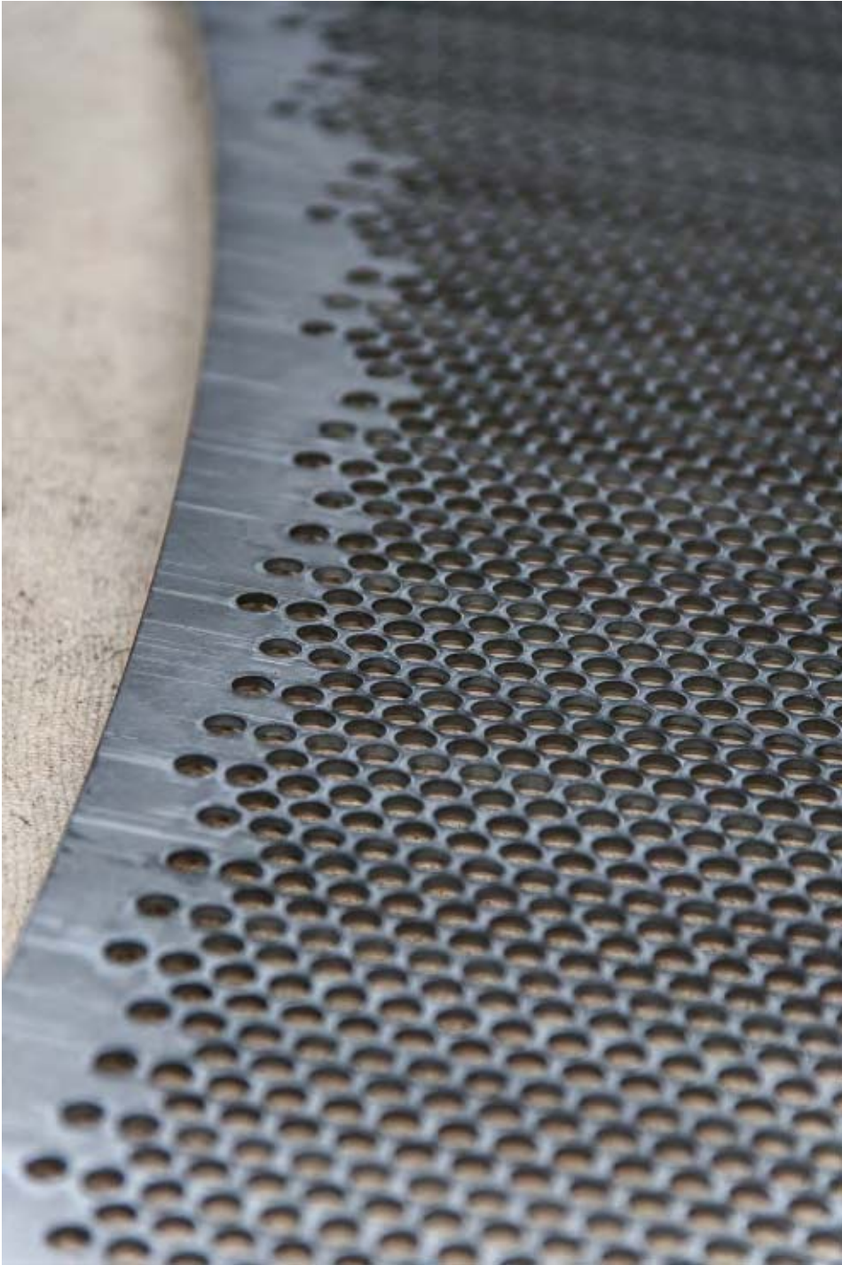
Best Practice: Perforated plates with continuous margins
