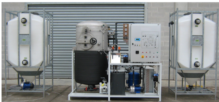
Small evaporator With storage tanks.
