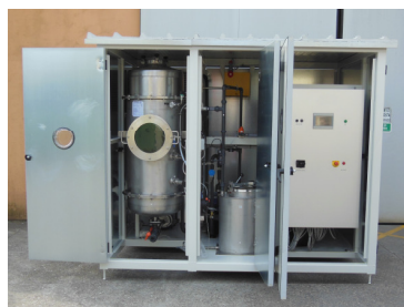
Small evaporator In enclosure with active carbon filter.
