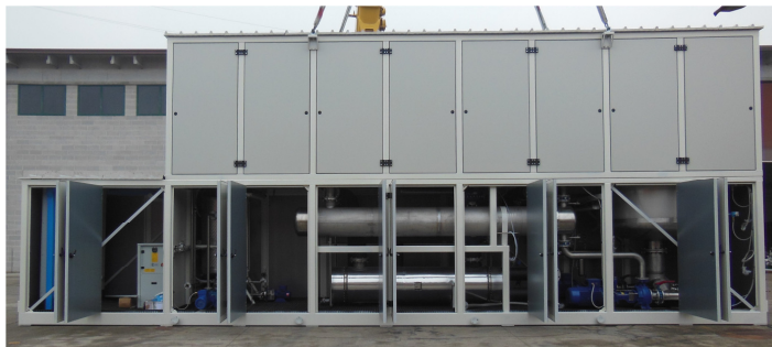
Evaporator built in a special container.
