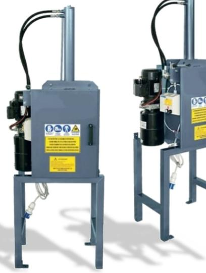
The MG5TFL drum crusher is ideal for crushing any type of can up to 30 litre capacity. A drain with hose is provided in the centre of the crush chamber to allow collection of liquid residues in a drum. The unit is operated by a control lever to lower and raise the crushing plate.
