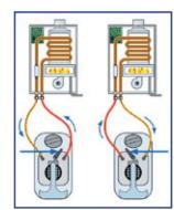
Always wash out the pump after use by circulating clean water through it, to remove any residues of the descaling solution.
