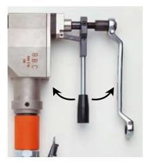
Lever handle for feeding the cutter head in tight spots where manual feeding is impossible.
