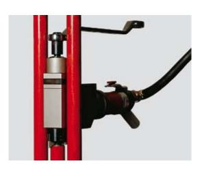
Pipe beveler MINI C40, pneumatic version, with 40mm body and cutter head for jobs in extremely restricted access areas.
