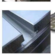
The PR/F modules are equipped with embedded "T" slots sono to fix the polar extensions and additional bigger "T" slots for mechanical fixtures or additional tools.
