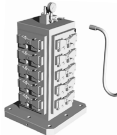
Blank system + hydraulics. Hydraulic connection is uncoupled after loading. Used in FMS systems.
