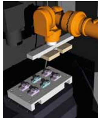
Grid System + hydraulics. Continuous hydraulic connection with vertical machining center.
