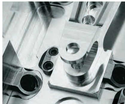
The support surface of the Dyna-Force® clamp can be installed flush with the fixture plate or raised to hold the workpiece off the fixture, enabling drill through.
