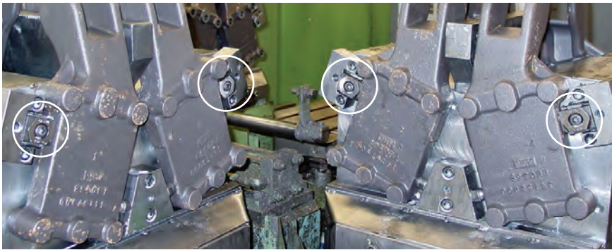
Up to 33,000 lbs. of clamping force allowing full capabilities of machine and tooling components
