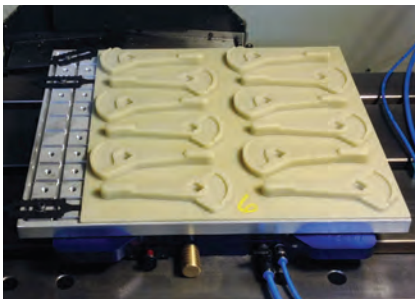
Workpiece placed over gasket to create a vacuum. Sliding stops used for location. (VM300 Vacuum Pallet - 45150)
