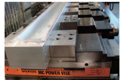
▲ Long-size precision equipment parts are machined.
