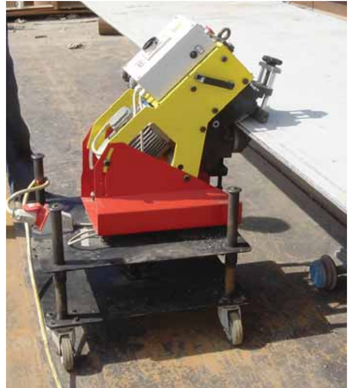
The Challenge 15 once mounted onto the plate edge will propel itself along automatically without any operator intervention
