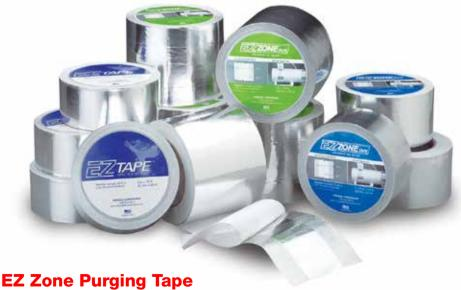
Used to seal root gaps and entrap the purging gas in the weld chamber. The tape has adhesive edges and an adhesive free centre strip so the adhesive never interferes in the welding process. Halogen and fluorocarbon free.
