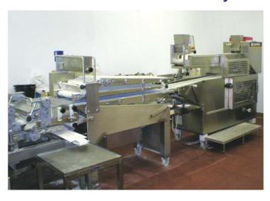
Investment in a new bakery is part of Graham Whitely's plan for the future of Superior Sandwiches, Widnes. Eurobake and Superior Sandwiches worked together to develop the bakery to meet expansion requirements for the future, installing a Kemper Mini Quadro Round Roll Plant with resting station and pinner, Kemper Relaxer, two Mondial Freddo Retarders and a Mondial Forni Rack Oven to create an integrated system.
